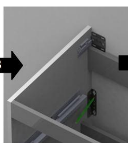
3 Marquer les trous des pattes de fixation Mark the holes of the additional support brackets
