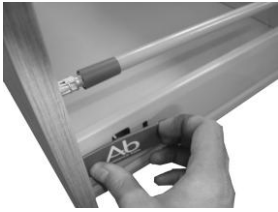
1/ Removing lateral cover
